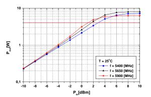
Saturation characteristic (frequency as parameter).
