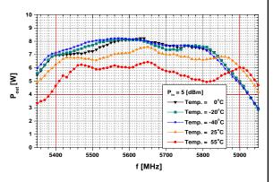
Output power vs. frequency (temperature as parameter).
