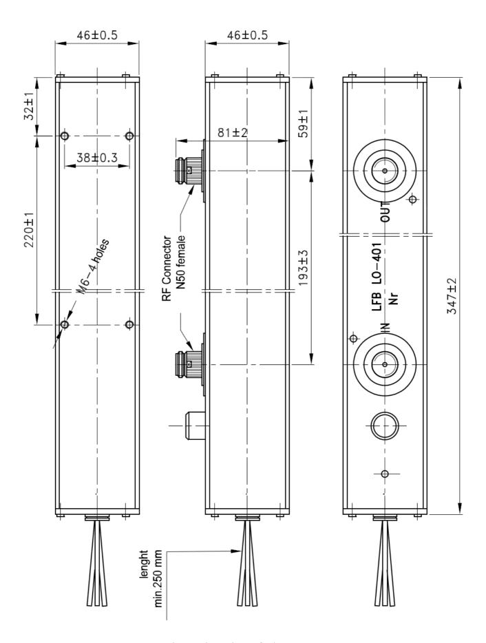
Fig. 2. Dimensions of tube LO-401
