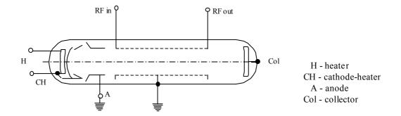
Fig. 1. Scheme connections of electrodes tube LO-401
